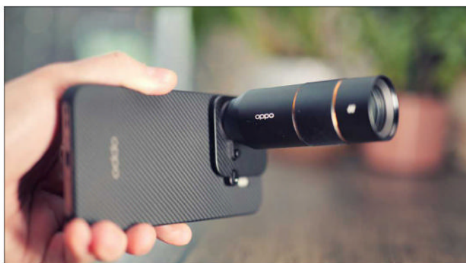
The teleconverter lens attaches via a small bayonet mount on a plate, which slides over the camera module and clicks into place.
